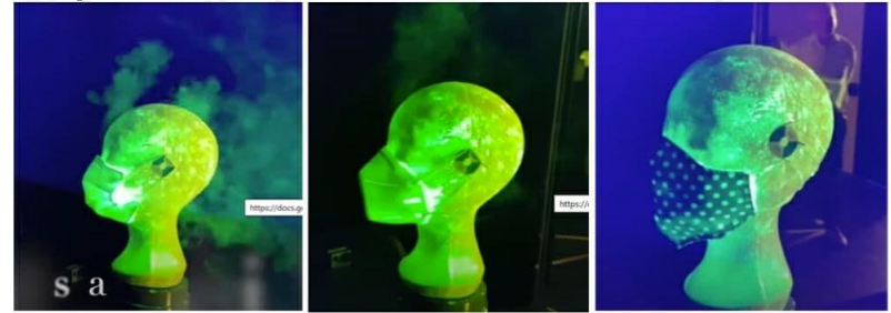
Figure: stills from mask visualization video showing leaks around gaps, which are major for the mask on the left, small for the mask in the middle, and not visible for the mask on the right.
